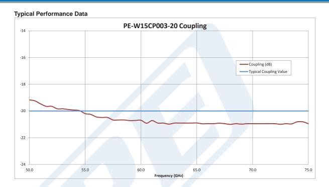
Click the following link (or enter part number in "SEARCH" on website) to obtain additional part information including price, inventory and certifications: WR-15 20 dB Directional Waveguide Coupler With UG-385/U Flange and E-Plane Coupled Port From 50 GHz to 75 GHz V Band PE-W15CP003-20
