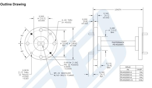
WR-22 Instrumentation Grade Straight Waveguide Section 6 Inch Length with UG-383/U Flange Operating from 33 GHz to 50 GHz from Pasternack Enterprises has same day shipment for domestic and International orders. Our RF, microwave and millimeter wave products maintain a 99% availability and are part of the broadest selection in the industry.
