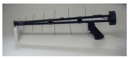
elements that fold into a storage tube. A thumb button releases a fold down pistol grip handle that locks the antenna into the storage tube. The storage tube has a collar at the top for an 8 foot adjustable strap that allows for over the shoulder or waist line attachment.
