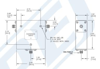
50 Ohm SMA Circulator Operating From 1.7 GHz to 2.2 GHz And 10 Watts With 18 dB Isolation from Pasternack Enterprises has same day shipment for domestic and International orders. Our RF, microwave and fiber optic products maintain a 99% availability and are part of the broadest selection in the industry.
