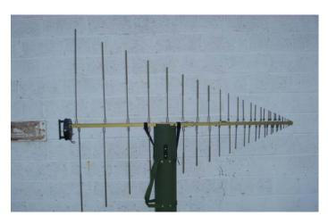
for use in environments found around the world. The complete assembly breaks into two main parts with elements that collapse and fold down. The antenna is supplied in a fiberglass storage tube that can be used as a mount.
