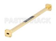
WR-28 Instrumentation Grade Straight Waveguide Section 9 Inch Length with 599/U Flange Operating from 26.5 GHz to 40 GHz
