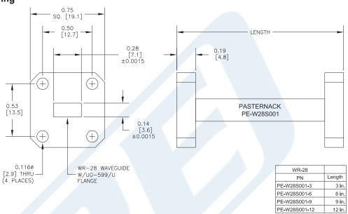
WR-28 Instrumentation Grade Straight Waveguide Section 6 Inch Length with 599/U Flange Operating from 26.5 GHz to 40 GHz from Pasternack Enterprises has same day shipment for domestic and International orders. Our RF, microwave and millimeter wave products maintain a 99% availability and are part of the broadest selection in the industry.
