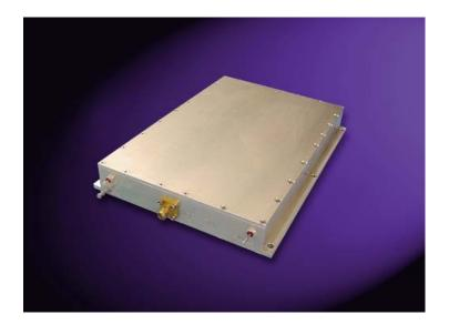
housing size is approximately 4.75 X 7.25 X 1.00 inches not including the mounting flange. The mounting flange runs along the both sides of the length dimension of 7.25" and employs six through holes for mounting to a heat sink. SMA female connectors are standard in the RF input and output ports. DC, command/control signals are accessible via DC feed through capacitors.
