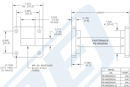
WR-62 Instrumentation Grade Straight Waveguide Section 9 Inch Length with UG-419/U Flange Operating from 12.4 GHz to 18 GHz from Pasternack Enterprises has same day shipment for domestic and International orders. Our RF, microwave and millimeter wave products maintain a 99% availability and are part of the broadest selection in the industry.
