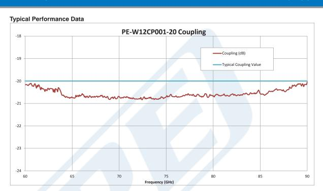
Click the following link (or enter part number in "SEARCH" on website) to obtain additional part information including price, inventory and certifications: WR-12 20 dB Directional Waveguide Coupler With UG-387/U Flange and H-Plane Coupled Port From 60 GHz to 90 GHz E Band PE-W12CP001-20
