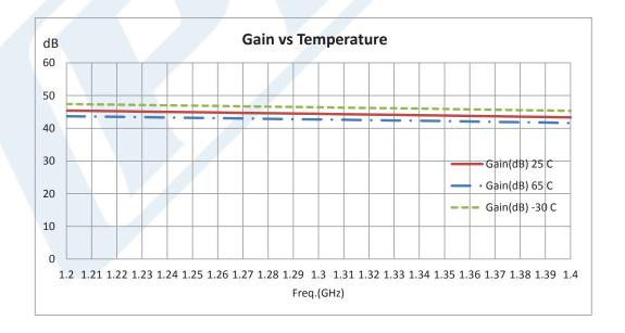
Click the following link (or enter part number in "SEARCH" on website) to obtain additional part information including price, inventory and certifications: 40 dB Gain, 10 Watt, 1.2 GHz to 1.4 GHz, High Power High Gain Amplifier, SMA PE15A5001
