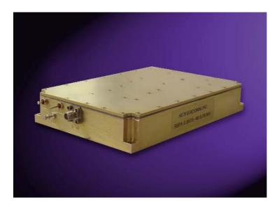
This SSPA is ideal for S Band Communication/Telemetry Systems that require high reliability, excellent linearity and high power in a rugged and compact module. Standard housing size is approximately 4.000(w) X 6.000(l) X 1.018(h) inches. Mounting is accomplished via four through holes in the housing. An SMA female connectors is standard on the RF input port. An SMA female connector is standard on the output port. DC connections are accessible via DC feed through capacitors.
