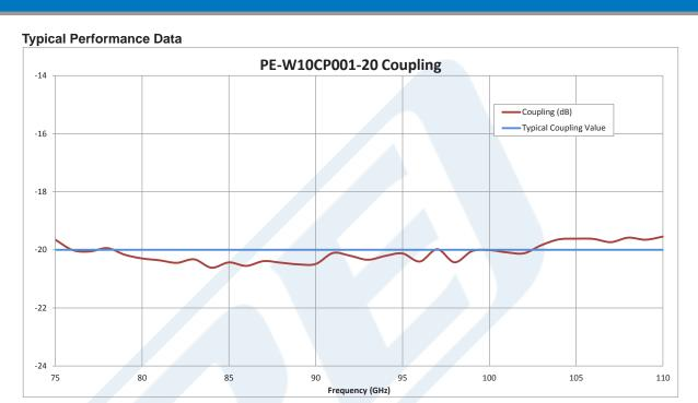
Click the following link (or enter part number in "SEARCH" on website) to obtain additional part information including price, inventory and certifications: WR-10 20 dB Directional Waveguide Coupler With UG 387/U-Mod Flange and H-Plane Coupled Port From 75 GHz to 110 GHz W Band PE-W10CP001-20
