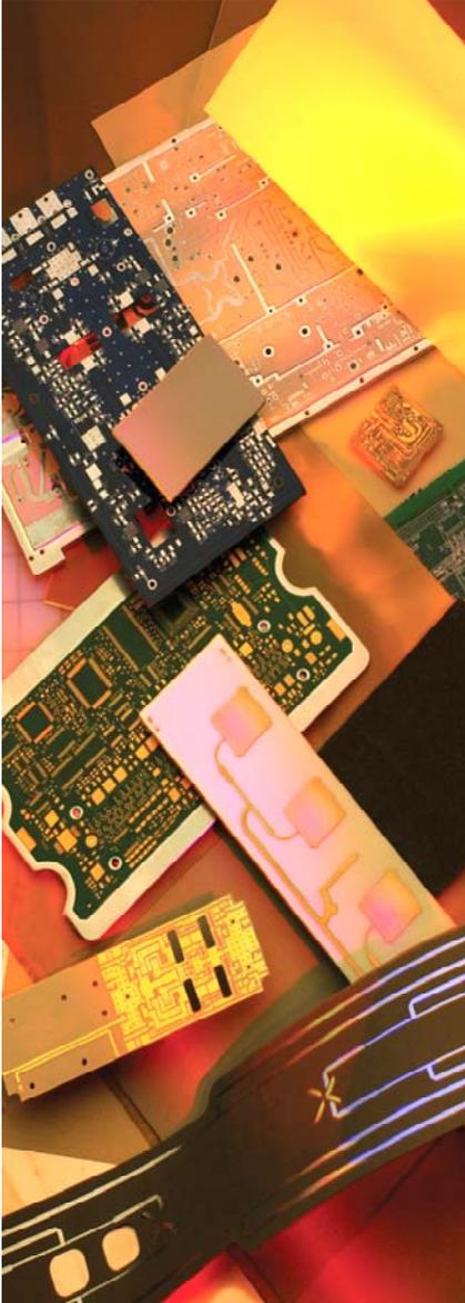
85NT is a pure polyimide laminate and prepreg system ( $T_g = 250^\circ\text{C}$ ), reinforced with a non-woven aramid substrate. This system combines the high-reliability features of polyimide (improved PTH reliability and temperature stability) with the low in-plane (x,y) expansion and outstanding dimensional stability of a non-woven aramid reinforcement.
