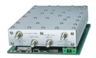
The SC5406A also has a wide gain range. Output signal levels as low as -110 dBm and as high as +16 dBm can be achieved.
