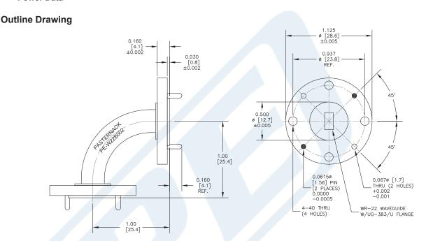
WR-22 Instrumentation Grade Waveguide H-Bend with UG-383/U Flange Operating from 33 GHz to 50 GHz from Pasternack Enterprises has same day shipment for domestic and International orders. Our RF, microwave and millimeter wave products maintain a 99% availability and are part of the broadest selection in the industry.
