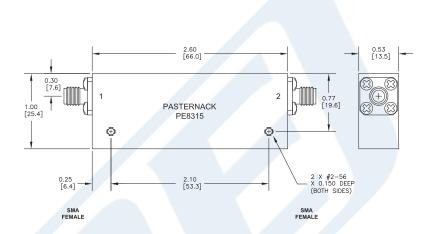
50 Ohm SMA Isolator Operating From 4 GHz to 18 GHz And 10 Watts With 15 dB Isolation from Pasternack Enterprises has same day shipment for domestic and International orders. Our RF, microwave and fiber optic products maintain a 99% availability and are part of the broadest selection in the industry.
