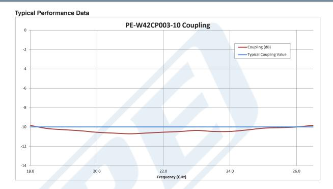
Click the following link (or enter part number in "SEARCH" on website) to obtain additional part information including price, inventory and certifications: WR-42 10 dB Directional Waveguide Coupler With UG595/U Flange and E-Plane Coupled Port From 18 GHz to 26.5 GHz K Band PE-W42CP003-10
