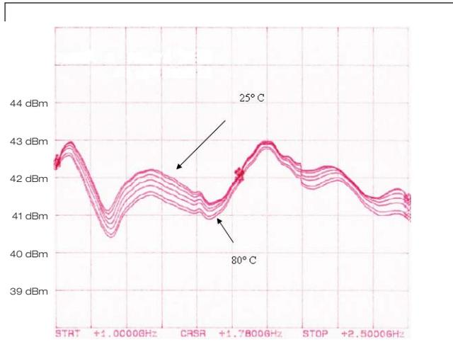
Small Signal Gain DATA from 25°C to 80°C Base Plate
