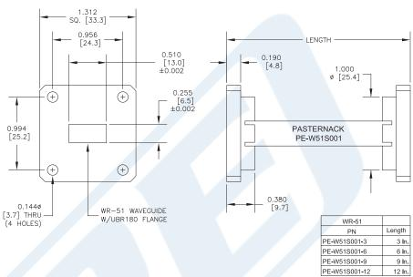
WR-51 Instrumentation Grade Straight Waveguide Section 9 Inch Length with R180 Flange Operating from 15 GHz to 22 GHz from Pasternack Enterprises has same day shipment for domestic and International orders. Our RF, microwave and millimeter wave products maintain a 99% availability and are part of the broadest selection in the industry.
