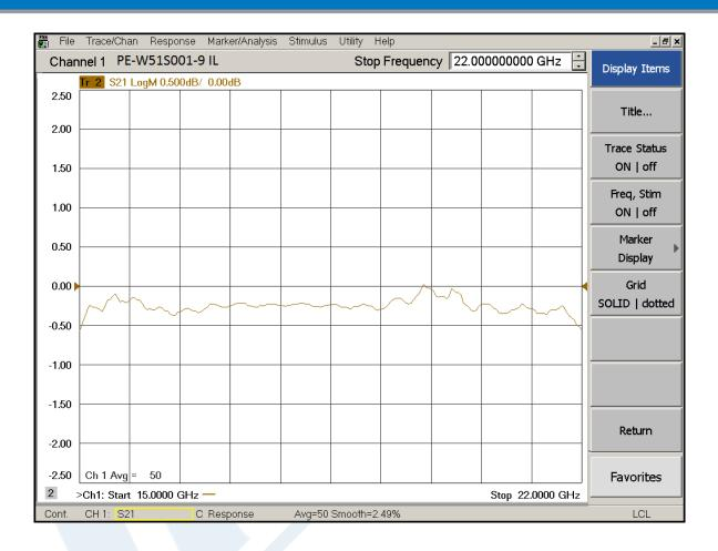
Click the following link (or enter part number in "SEARCH" on website) to obtain additional part information including price, inventory and certifications: WR-51 Instrumentation Grade Straight Waveguide Section 9 Inch Length with R180 Flange Operating from 15 GHz to 22 GHz PE-W51S001-9
