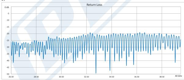
Click the following link (or enter part number in "SEARCH" on website) to obtain additional part information including price, inventory and certifications: WR-28 Flexible Waveguide Twist With a UG-599/U Flange Operating From 26.5 GHz to 40 GHz PE-W28TF005-24
