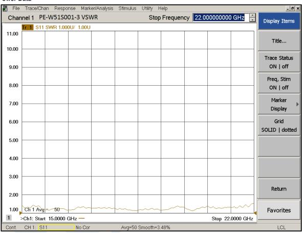
Click the following link (or enter part number in "SEARCH" on website) to obtain additional part information including price, inventory and certifications: WR-51 Instrumentation Grade Straight Waveguide Section 3 Inch Length with R180 Flange Operating from 15 GHz to 22 GHz PE-W51S001-3
