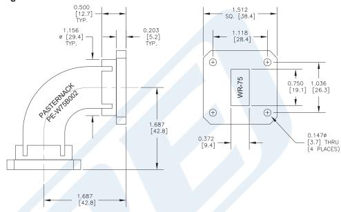
WR-75 Waveguide H-Bend with WR-75-BR-MB Flange Operating from 10 GHz to 15 GHz from Pasternack Enterprises has same day shipment for domestic and International orders. Our RF, microwave and millimeter wave products maintain a 99% availability and are part of the broadest selection in the industry.
