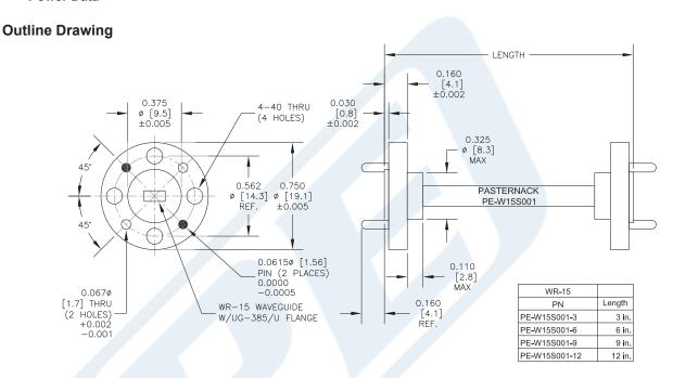
WR-15 Instrumentation Grade Straight Waveguide Section 3 Inch Length with UG-385/U Flange Operating from 50 GHz to 75 GHz from Pasternack Enterprises has same day shipment for domestic and International orders. Our RF, microwave and millimeter wave products maintain a 99% availability and are part of the broadest selection in the industry.
