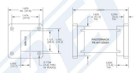
WR-112 Commercial Grade Straight Waveguide Section 3 Inch Length with UG-51/U Flange Operating from 7.05 GHz to 10 GHz from Pasternack Enterprises has same day shipment for domestic and International orders. Our RF, microwave and millimeter wave products maintain a 99% availability and are part of the broadest selection in the industry.
