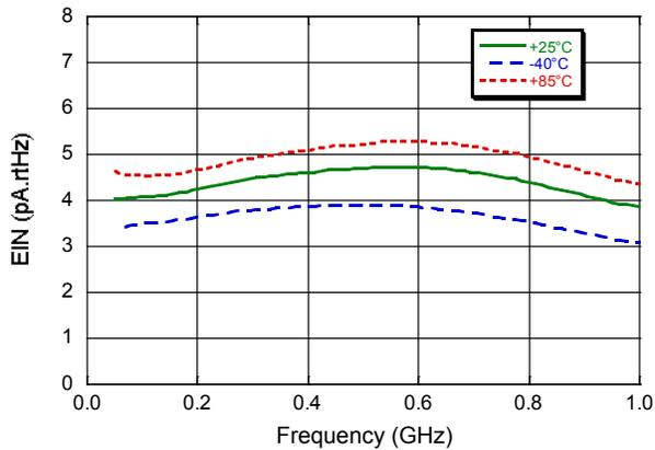
**Typical Performance Curves: 79 Channels; NTSC Frequency Plan,  $P_{OUT} = 20 \text{ dBmV/ch}$**
