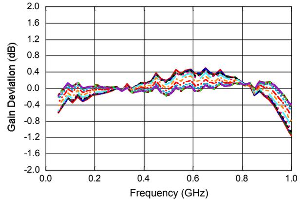
**Gain vs. Frequency to 1.6 GHz @ +25°C**
