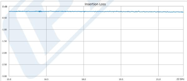
Click the following link (or enter part number in "SEARCH" on website) to obtain additional part information including price, inventory and certifications: WR-51 Flexible Straight Waveguide Section 12 Inch Length with Square Cover Flange Operating from 15 GHz to 22 GHz PE-W51SF005-12
