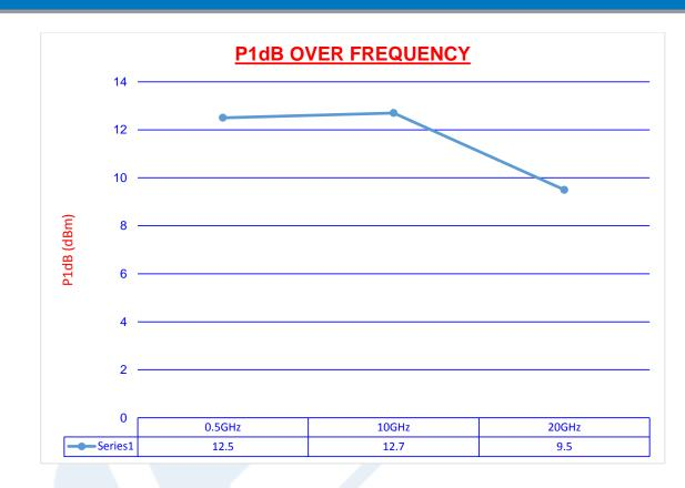
10 dBm P1dB, 50 MHz to 18 GHz, USB Controlled Broadband Amplifier, 12 dB Gain, 4.5 dB NF, SMA from Pasternack Enterprises has same day shipment for domestic and International orders. Our RF, microwave and millimeter wave products maintain a 99% availability and are part of the broadest selection in the industry.
