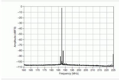
Two Tone Spectrum at 2 dBm Each, Bandpass Path, 4 kHz RBW
