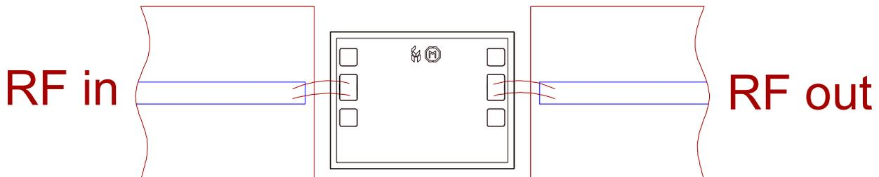
**GaAs MMIC devices are susceptible to damage from Electrostatic Discharge. Proper precautions should be observed during handling, assembly and test.**
