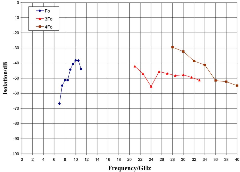
Output Spectrum @ +15 dBm Drive Level,  $T_A = 25\text{ }^\circ\text{C}$
