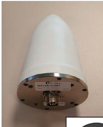
GPS Timing Antenna with Receiver (top); bottom view (inset)
