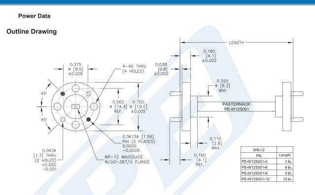
WR-12 Instrumentation Grade Straight Waveguide Section 6 Inch Length with UG-387/U Flange Operating from 60 GHz to 90 GHz from Pasternack Enterprises has same day shipment for domestic and International orders. Our RF, microwave and millimeter wave products maintain a 99% availability and are part of the broadest selection in the industry.
