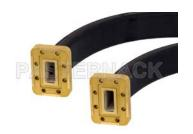
WR-90 Flexible Straight Waveguide Section 24 Inch Length with CPR-90G Flange Operating from 8.2 GHz to 12.4 GHz
