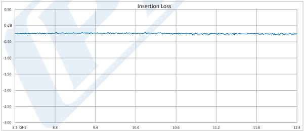
Click the following link (or enter part number in "SEARCH" on website) to obtain additional part information including price, inventory and certifications: WR-90 Flexible Straight Waveguide Section 24 Inch Length with CPR-90G Flange Operating from 8.2 GHz to 12.4 GHz PE-W90SF006-24
