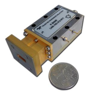
This Ka-Band Low Noise Amplifier (LNA) is designed to meet the extended K-Band Satcom bands and is ideally suited for airborne or SWaP applications where size weight and power are critical.
