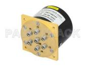
SP6T Electromechanical Relay Latching Switch DC to 40 GHz, 2.92mm, 3 Watts, 28V Control, Self Cut Off, Reset, Diodes
