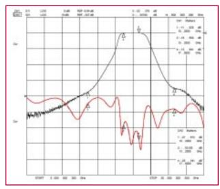
Forward Transmission (S21) and **Input Matching (S11)** characteristics
