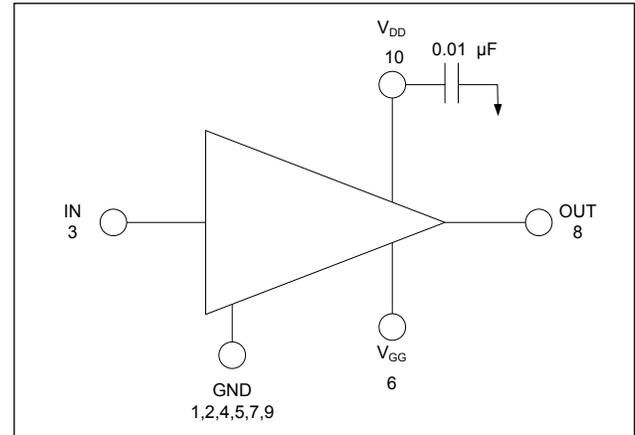
3. Nominal bias is obtained by first connecting  $-5$  volts to pin 6 ( $V_{GG}$ ), followed by connecting  $+8$  volts to pin 10 ( $V_{DD}$ ). Note sequence.
