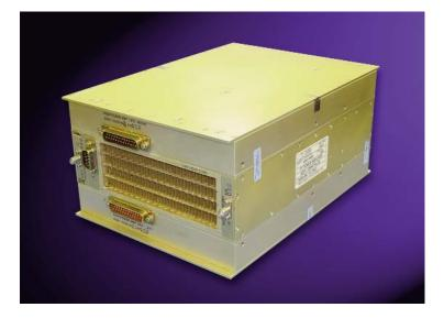
width monitor to protect the HPA in case the pulse width exceeds a predetermined level. The output has an isolator for protection and all the supplies are protected from over voltage and over current.
