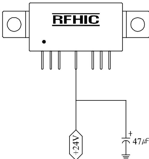
1. On the power input port (Pin#5), 47uF/35V capacitor GND is recommended.
