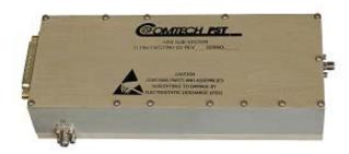
Comtech PST has announced the release of a solid state Class "AB" linear amplifier which operates over the full 2500-6000 MHz frequency band and delivers a minimum of 50 watts. The amplifier uses the latest Gallium Nitride (GaN) technology and is housed in a relatively small package measuring only 7.5" x 3.0" x 1.5" (excluding connectors).
