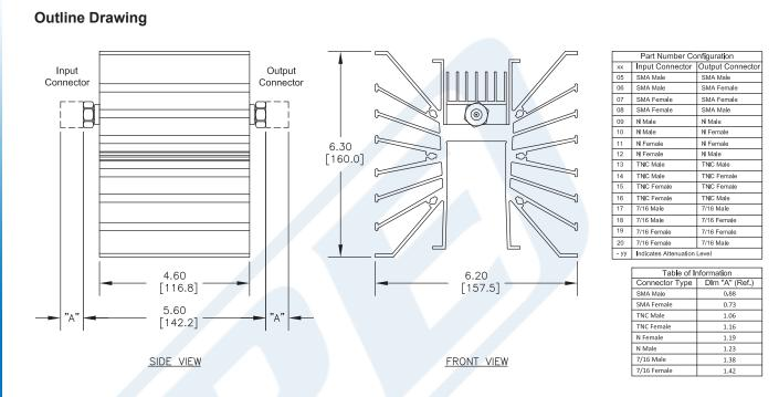
40 dB Fixed Attenuator, TNC Female To TNC Male Directional Black Aluminum Heatsink Body Rated To 300 Watts Up To 3 GHz from Pasternack Enterprises has same day shipment for domestic and International orders. Our RF, microwave and millimeter wave products maintain a 99% availability and are part of the broadest selection in the industry.
