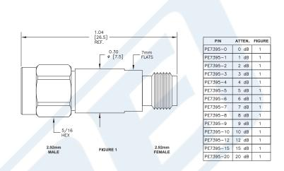
4 dB Fixed Attenuator, 2.92mm Male To 2.92mm Female Passivated Stainless Steel Body Rated To 2 Watts Up To 40 GHz from Pasternack Enterprises has same day shipment for domestic and International orders. Our RF, microwave and millimeter wave products maintain a 99% availability and are part of the broadest selection in the industry.
