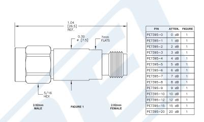
15 dB Fixed Attenuator, 2.92mm Male To 2.92mm Female Passivated Stainless Steel Body Rated To 2 Watts Up To 40 GHz from Pasternack Enterprises has same day shipment for domestic and International orders. Our RF, microwave and millimeter wave products maintain a 99% availability and are part of the broadest selection in the industry.
