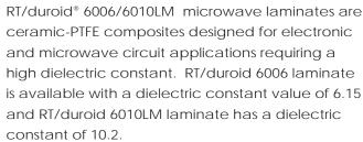
RT/duroid 6006/6010LM microwave laminates feature ease of fabrication and stability in use. They have tight dielectric constant and thickness control, low moisture absorption, and good thermal mechanical stability.
