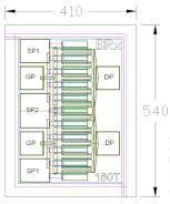
$\begin{array}{l} \mbox{Chip dimensions}: 410 \ X \ 540 \ microns\\ \mbox{Gate pad}(GP): 75 \ X \ 75 \ microns\\ \mbox{Drain pad}(DP): 75 \ X \ 75 \ microns\\ \mbox{Source pad}(SP1): 95 \ X \ 75 \ microns\\ \mbox{Source pad}(SP2): 95 \ X \ 110 \ microns\\ \mbox{Chip thickness}: 100 \ microns\\ \end{array}$
