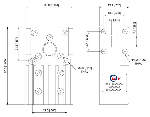
Unit: mm/ inch, General part tolerance is ±0.2mm unless otherwise stated.
