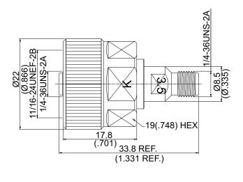
Note:Ruggedized K jack to be mounted directly on vector network analyzer.
