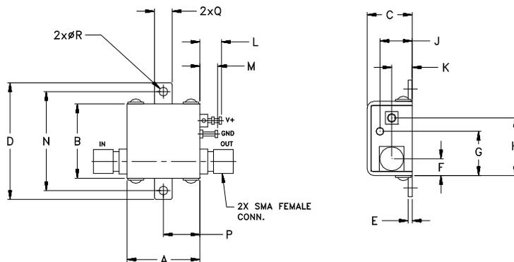
**!** NOTE: When soldering the DC connections, caution must be used to avoid overheating the DC terminals. See Application Note [AN-40-10](#).
