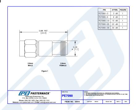
10 dB Fixed Attenuator, 2.92mm Male To 2.92mm Female Passivated Stainless Steel Body Rated To 2 Watts Up To 40 GHz from Pasternack Enterprises has same day shipment for domestic and International orders. Our RF, microwave and millimeter wave products maintain a 99% availability and are part of the broadest selection in the industry.
