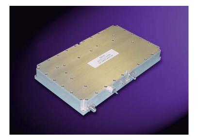
inches. Mounting is accomplished via six through holes in the housing. An SMA female connectors is standard on the RF input port. An SMA male connector is standard on the output port. DC connections are accessible via a DC feed through capacitor. The TTL Switching command is applied via an SMC male connector.
